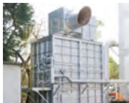
Secondary Combustion Furnace
