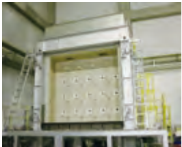
Structural Fire resistance Furnace (Large scale, for Walls)
