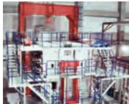
Structural Fire resistance Furnace (Large scale, for Beams, Slabs and Columns)
