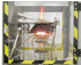
Cone Calorimeter (ISO 5660)
