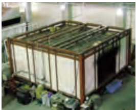
Full-Scale Compartment for Fire Experiment (with Water Pump)
