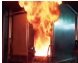
Room Corner Testing Unit (ISO 9705)
