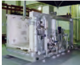
Structural Fire resistance Furnace (Medium scale)
